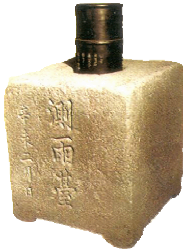
Figure 1. The world's first rain gauge. It was developed in 1442 by King Sejong the Great and used since that time. It was distributed to local governments under the direct supervision of the King. Rainfall data thus measured were gathered through a nationwide network and records were kept for more than 500 years after its development.
